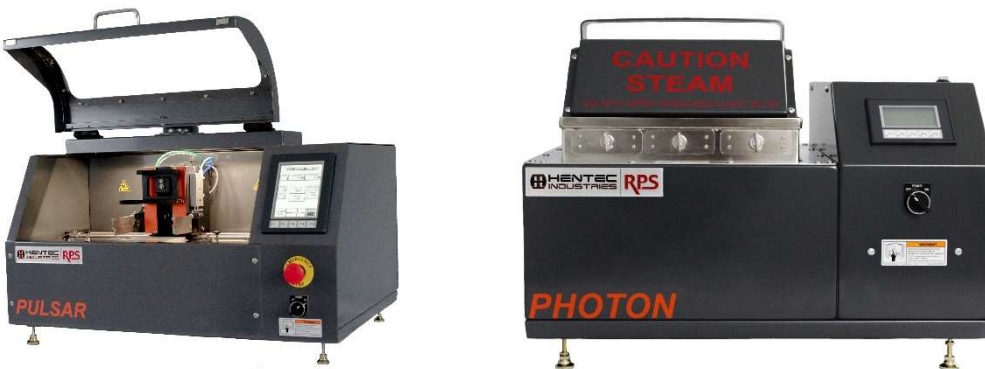
Figure 6: Dip-and-look solderability test equipment (left), and component steam aging system (right)
