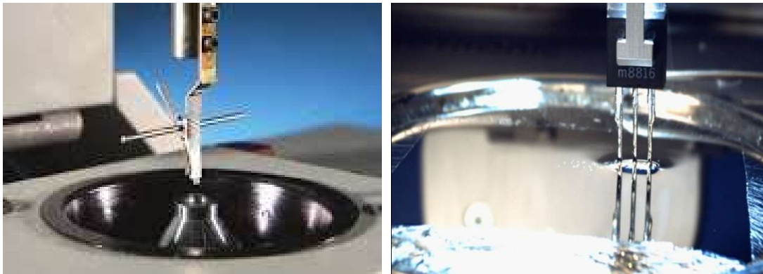
Figure 1. Wetting balance solderability test system (left), and dip-and-look solderability test system (right)
