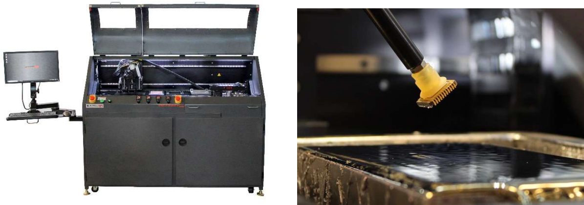
Figure 5. Odyssey 1325 lead tinning system (left), quad flat pack (QFP) device during re-tinning (right)
