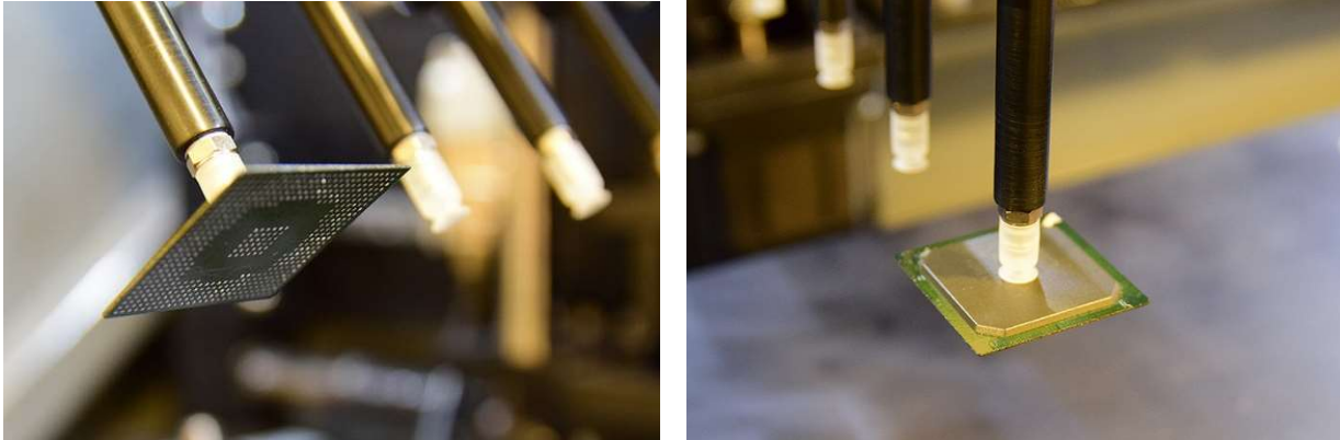
Figure 6. Ball grid array device before de-balling (left), and ball grid array being de-balled (right)
