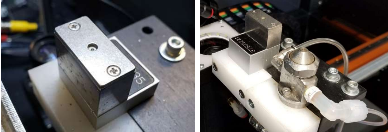
Figure 3. Drop-jet flux dispenser (left), and dual spray and drop-jet fluxing system (right)
