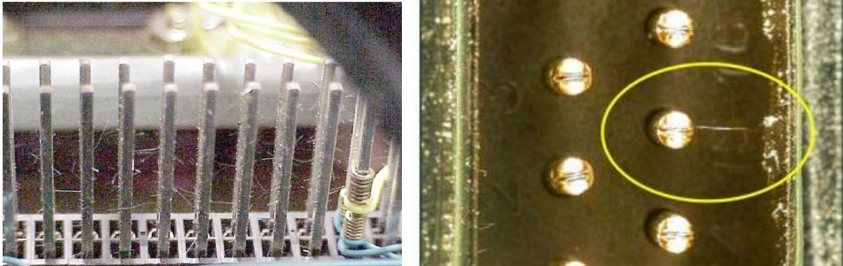
Figure 2. Tin whisker growth from plated leads (left), and electrical short resulting from tin whisker (right)
