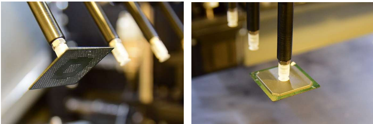
Figure 3. Ball grid array device before de-balling (left), and ball grid array being de-balled (right)
